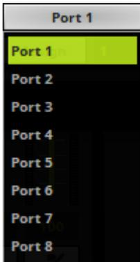
**Port** - Defines the port [Port 1 - 8] that is assigned to this DMX-IN Device. MADRIX 5 allows you to send trigger signals from up to 8 different devices [8 ports] and assign a MADRIX 5 TRI Effect the corresponding port.
