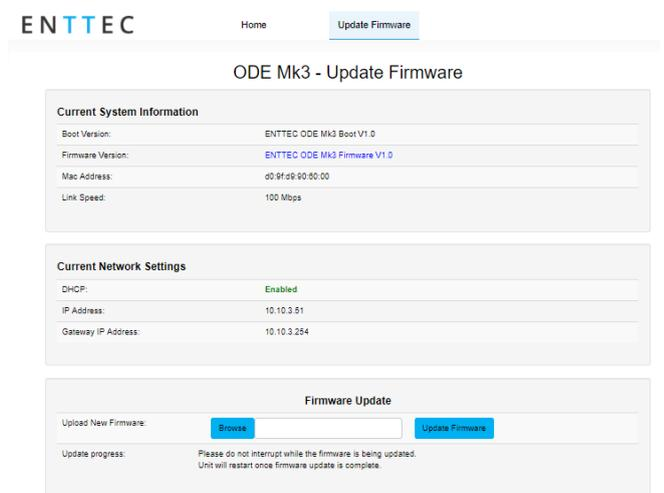
After the update has completed, the web interface will load the Home tab, where you can check the update was successful under Firmware Version. Once the Home tab has loaded, the ODE MK3 will resume operation.
