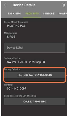
9. The PILOTINO™ PCB will be automatically restored to its factory default settings.
