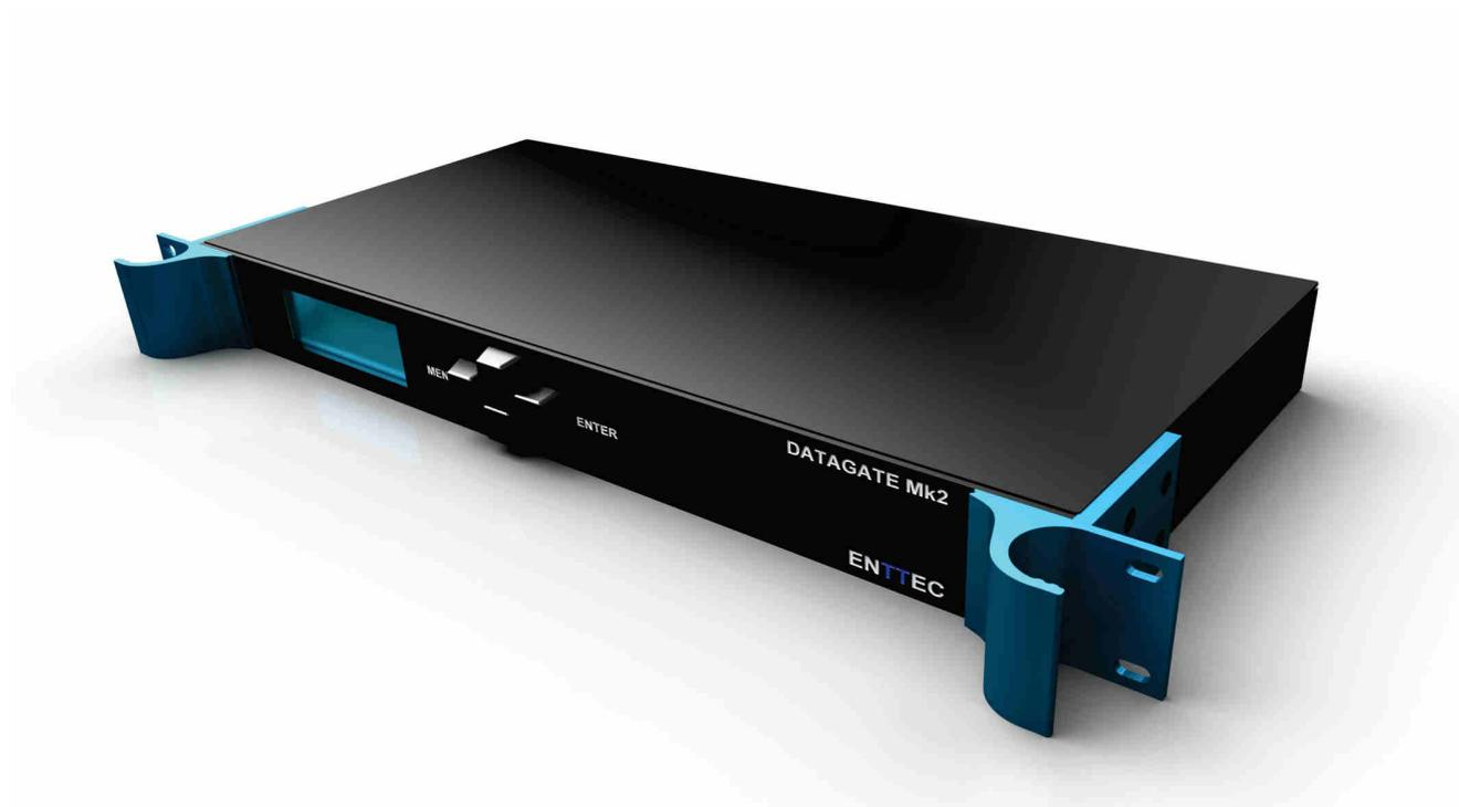
The Datagate is an extremely powerful and flexible bridge between controls and any DMX512 device. It can form the backbone of a network, provide optical isolation, merge levels from multiple streams, translate between DMX and Ethernet protocols and even play back Architectural lighting shows.
