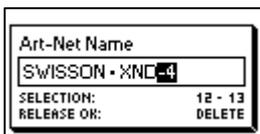
Then keep [OK] pressed and turn the encoder clockwise until all of the text that you wish to delete appears highlighted.
