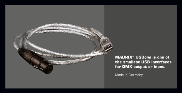
The MADRIX® USB*one* allows you to control 512 DMX channels using the MADRIX® software. Mainly used for DMX input, an additional MADRIX® KEY (a software license) is required for DMX output.
