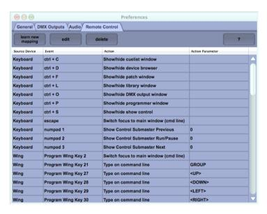
You can remotely control certain features of DMXIS Pro using external control surfaces - including Enttec Wings, MIDI controllers or your computer keyboard.
