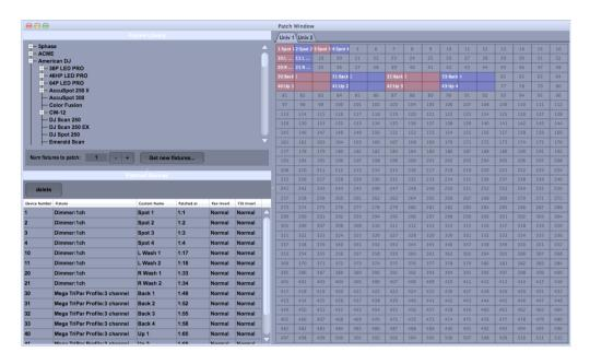
The top left is the Fixture Library panel, which lists all manufacturers and fixtures that are available for patching. These fixture profiles are stored locally on your computer. The "Get new fixtures..." button allows you to import extra manufacturers and fixtures into your D-Pro installation.
