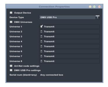
This example shows that Universe 1 data will be transmitted to the first available DMX USB Probox that is detected.
