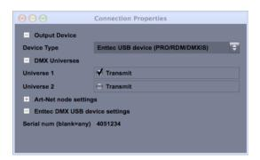
Double-click on a line to open the "Connection Properties" dialog, from where you can configure the connection – which universe(s) to transmit, the network settings (for Art-Net connections) or the hardware serial number (for USB devices).
