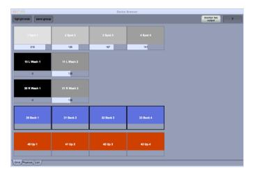
The grid tab is useful for large rigs with many conventional dimmers. Due to the grid layout, you can visualise and select many hundreds of channels easily. You can customise the number of devices displayed on each row from the Preferences window.
