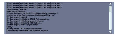
Under the window buttons is the terminal area. In here, you will see diagnostic and error messages relating to the current D-Pro session. Command line activity, and any output generated by Python FX scripts is also displayed here.
