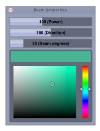
Every patched fixture in your rig – even plain dimmer channels – can display a virtual beam in the browser window. As the screenshot on the previous page shows, this is extremely useful for basic visualisation of fixed devices.
