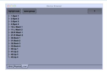
In the list tab, all devices are displayed as a simple flat list. Devices can be selecting by clicking, shift-clicking or ctrl-clicking. This tab does not display any attributes such as dimmer levels.
